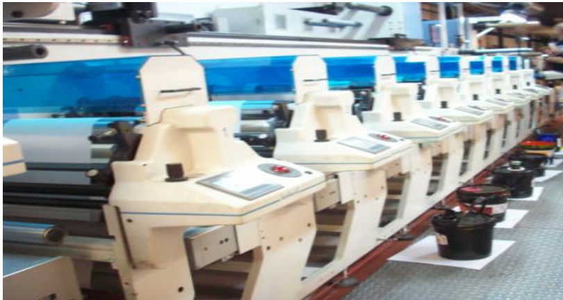
Xerography line capable to print 8 colours sequentially.
